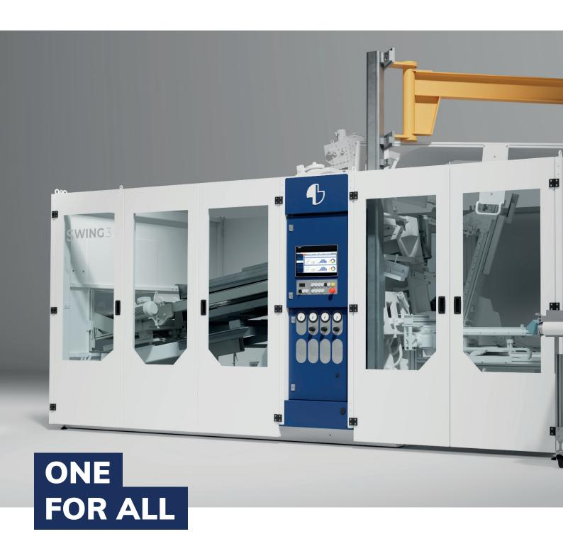
Compact, flexible and adjustable: The SWING is the perfect all-round system for the production of cups, trays, and lids.
